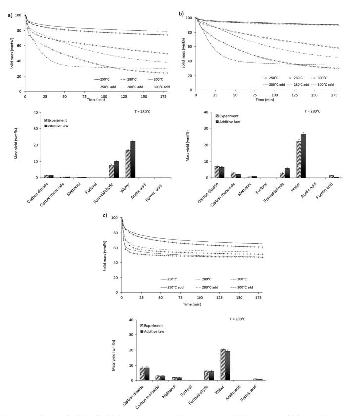
Fig. 5. Comparison between results obtained with additive law on single constituents and with mixtures a) cellulose—lignin; b) cellulose—xylan; c) lignin—xylan. Solid mass loss measured in TGA device is given versus time at three temperatures and volatile yields measured in TGRNADE are given at 280 °C after 180 min.
