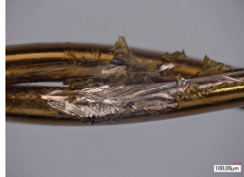
Fig. 4d. Heavy wound on the wire
