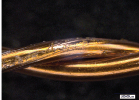
Fig. 4c. Medium wound on the outer part of the wire
