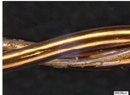
Fig. 4b. Medium wound on the inner part of the wire
