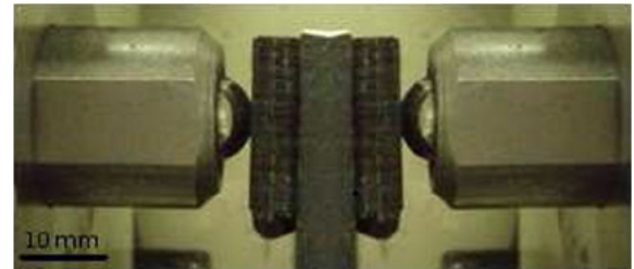
Fig. 11 – Image of the specimen composed of 2 C/C composite samples glued on a metallic substrate. (A colour version of this figure can be viewed online.)
