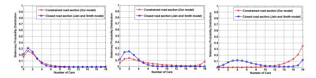
Figure 7: Stationary probability distributions.  $\lambda = 1000 \text{ veh/h}$ , 2000 veh/h and 3000 veh/h respectively from left to right sides.
