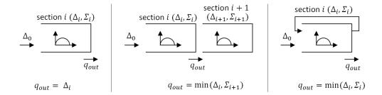
Figure 3: open, constrained and closed road section systems, respectively from left to right sides.
