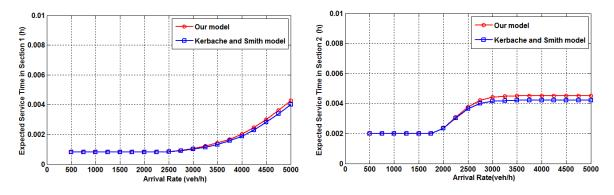
Figure 11: Comparison of the expected service time. In left, section 1. In right, section 2. In red color, our model of two sections in tandem. In blue color, open M/G/c/c state dependent queueing networks in tandem.
