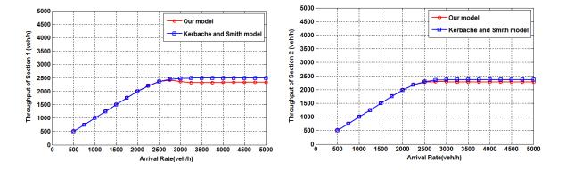
Figure 10: Comparison of the throughputs. In left, section 1 ( $\theta$ ). In right, section 2 ( $\sigma$ ). In red color, our model of two sections in tandem. In blue color, open M/G/c/c state dependent queueing networks in tandem
