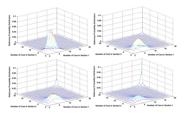
Figure 8: Stationary probability distribution of the number of cars in two road sections in tandem. The arrival rate  $\lambda = 1000 \text{ veh/h}$ , 2000 veh/h, 2500 veh/h and 3000 veh/h.
