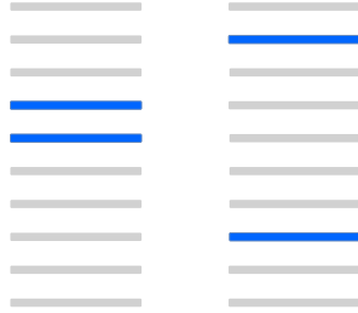
Fig. 1: Two rankings (with two positives and eight negatives examples) ordered from the highest score (at the top) to the lowest. On the left, we get AUCROC = 0.63 and AP = 0.33 . On the right, AUCROC = 0.56 and AP = 0.38 . Therefore, the two criteria disagree on the best ranked list.
