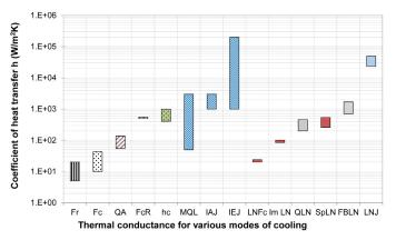
**Fig. 26.** Typical values of CHT in various cooling regimes. Fr: free convection in air/ GN. Fc: forced convection. QA: air quenched. FcR: on rotating parts in air. hc: thermal contact conductance. MQL: min. quantity lubrication. IAJ: impinging air jet. IEJ: impinging emulsion jet. LNFc: LN flowing on plate. ImLN: immersed in LN, QLN: quenched in LN, SpLN: splashed with LN, FBLN: film boiling in LN, LNJ: LN jet [122].
