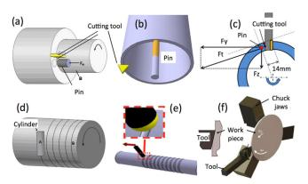
**Fig. 16.** Open tribometers for determining friction in cutting. Designed by (a) Olsson et al. [166], (b) Zemzemi et al. [229], (c) Smolenicki et al. [212], (d) Hedenqvist and Olsson [108], (e) Claudin et al. [60], (f) Puls et al. [180].
