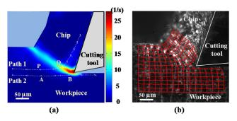
Fig. 2. PIV technique used to characterize deformation in machining: (a) Effective strain rate field, (b) Grid distortion [102].
