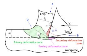
Fig. 1. Deformation zones in the metal cutting process.
