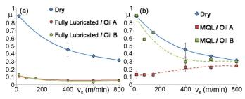
Fig. 19. Influence of lubrication and oil viscosity on friction: (a) full lubrication, (b) MQL [40].
