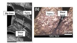
Fig. 30. Shear banding and twinning in (a) AISI 316L and (b) MgAZ31B chip [194,152].
