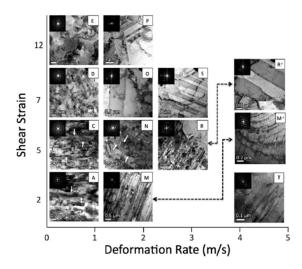
**Fig. 29.** Microstructures obtained in machining with varying rake angles and cutting speeds designed to yield differences in strain, strain rate and temperature [37].
