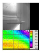
**Fig. 4.** Visible (top) and infrared temperature distribution in °C (bottom), obtained by high-speed videography of metal cutting (rectangle in visible image is  $\sim$ 0.3 mm horizontal infrared field of view) [117].
