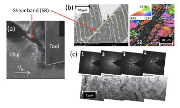
**Fig. 31.** Shear band characterization in machining using (a) PIV, (b) SEM/EBSD and (c) TEM. The far left panel in (c) represents microstructure in the centre of the shear band [193].
