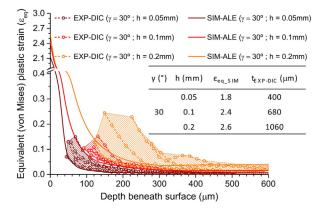
**Fig. 3.** Measured and predicted through-depth plastic strain distributions at different uncut chip thicknesses [167].
