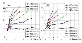
Fig. 21. Changes in friction coefficient at the (a) rake and (b) flank faces [98].
