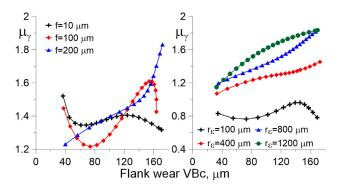
**Fig. 22.** Changes in the friction coefficient with tool wear due to variations in the (a) feed rate, and the (b) tool nose radius [93].
