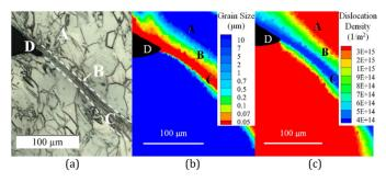
**Fig. 5.** (a) Optical micrograph of chip microstructure in the shear band, and simulated (b) grain size and (c) dislocation density distribution (cutting speed = 100 m/min, uncut chip thickness = 0.2 mm) [159].
