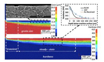
Fig. 32. Subsurface microstructure in machining Ti-6Al-4V [188].
