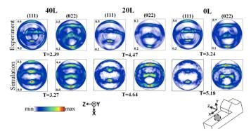
Fig. 33. Experimental and simulated orientation distribution functions for machining of copper [31].
