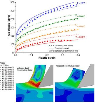
Fig. 10. Influence of constitutive model on the flow stress and machining simulations for OFHC copper [66].
