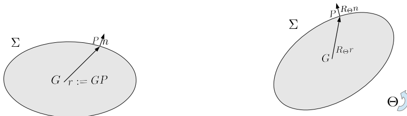
FIGURE 1. On the left, the reference rigid body \Sigma , on the right the rotated rigid body R_\Theta \Sigma
