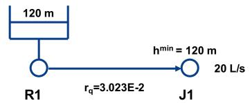
Figure 2. Network #1; one single pipe supplying the junction J1 with demand at d = 20 L/s from tank node R1; the tank is low and there is not enough pressure at J1.
