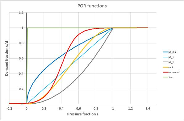
Figure 3. Examples of POR functions; the dark blue curve is the Wagner function; red is exponential; light blue and grey are power equations; yellow is cubic; and green is the step Heaviside function.
