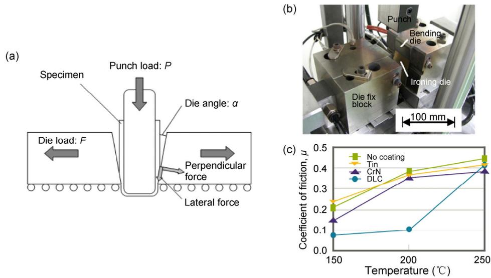
**Fig. 13** (a) Schematic of the U-bending-ironing tribometer; (b) U-bending-ironing apparatus; (c) friction coefficient of different coatings at different temperatures. Reproduced with permission from Ref. [78].
