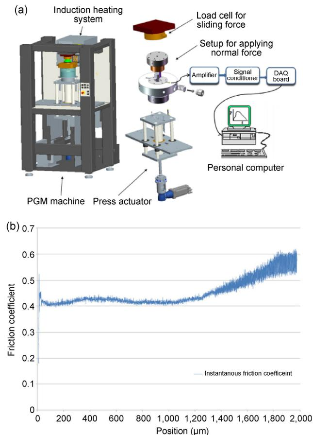
**Fig. 23** (a) Experimental setup of the modified sliding test; (b) instantaneous friction coefficient curve between a pair of steel-steel at 577 °C. Reproduced with permission from Ref. [88]. Copyright Elsevier, 2014.
