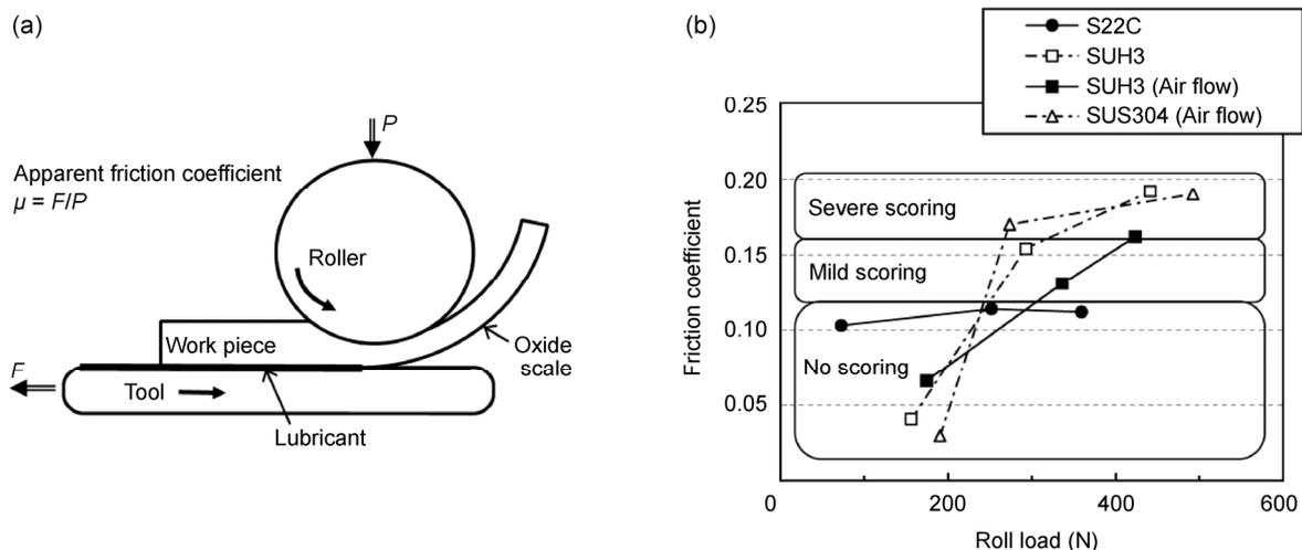
**Fig. 27** Tribometer for rolling developed by Iida and Hidaka: (a) schematic of the tribometer and (b) effects of rolling load on friction coefficient and scoring. Reproduced with permission from Ref. [90].
