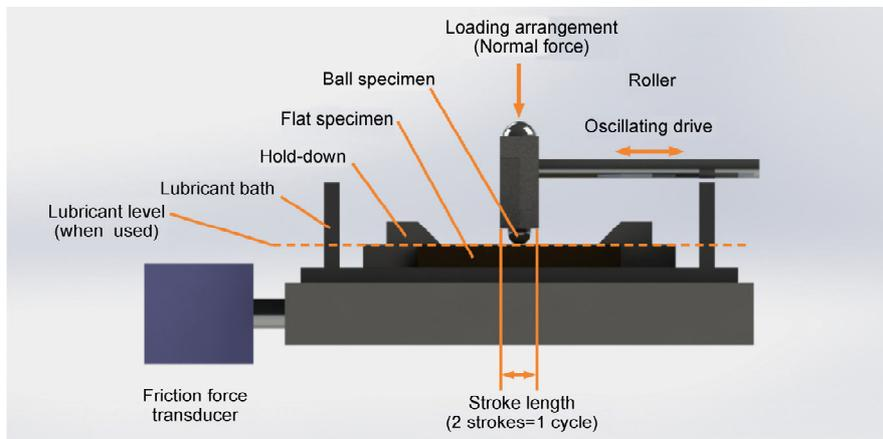
**Fig. 17** Schematic of ball-on-disc wear test system.
