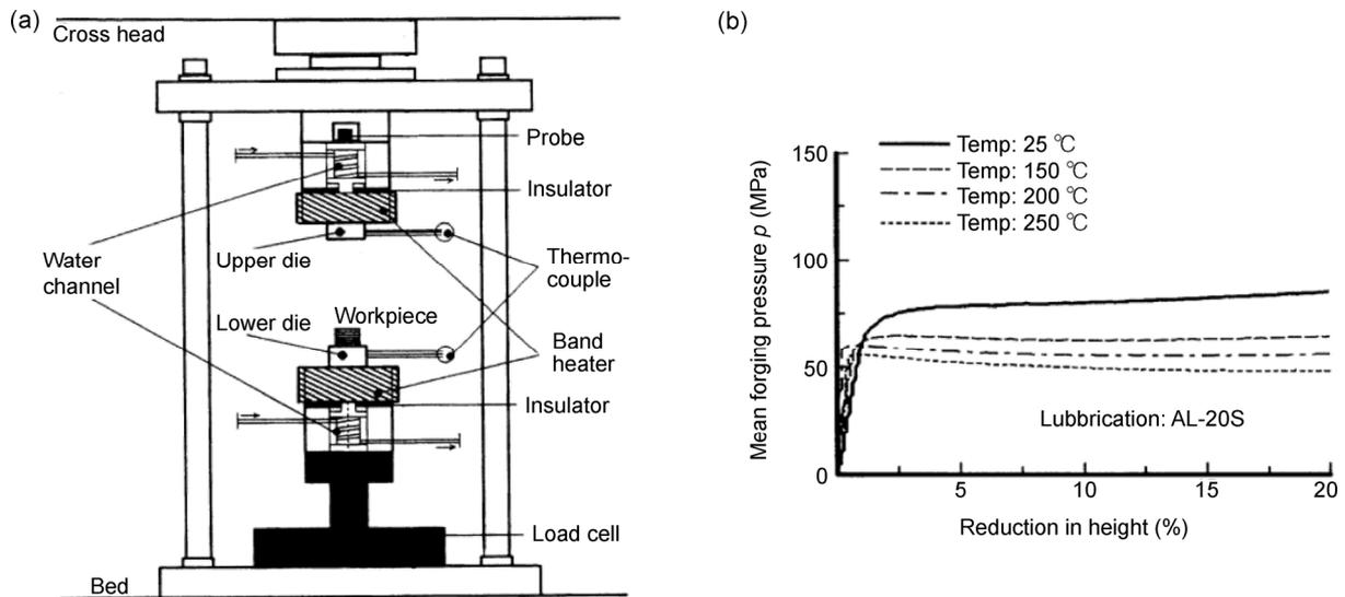
**Fig. 26** (a) Schematic of the ultrasonic reflection intensity evaluation test; (b) relationship between reduction in height and mean forging pressure (lubricated condition). Reproduced with permission from Ref. [89]. Copyright Elsevier, 2014.
