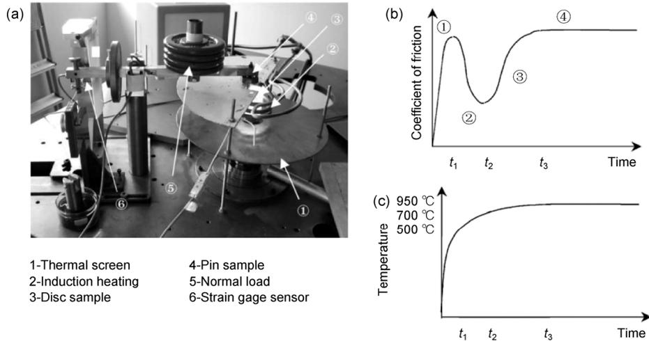
**Fig. 4** (a) High temperature pin-on-disc tribometer; (b) evolution of friction coefficient in the case of the non stabilized temperature in the pin; (c) evolution of the superficial temperature of the pin calculated by a numerical model. Reproduced with permission from Ref. [25]. Copyright Elsevier, 2014.
