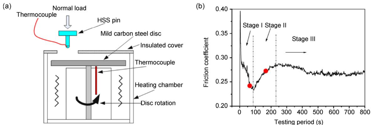
**Fig. 8** (a) Schematic of high temperature pin-on-disc test configuration; (b) three tribological stages and two interrupted points. Reproduced with permission from Ref. [75]. Copyright Elsevier, 2014.
