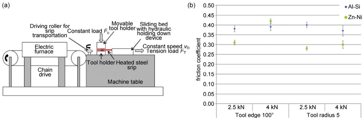
**Fig. 11** (a) Schematic representation of hot flat strip drawing simulator; (b) coefficients of friction for Al-Si and Zn-Ni coatings at different tested conditions in comparison. Reproduced with permission from Ref. [8]. Copyright Elsevier, 2014.
