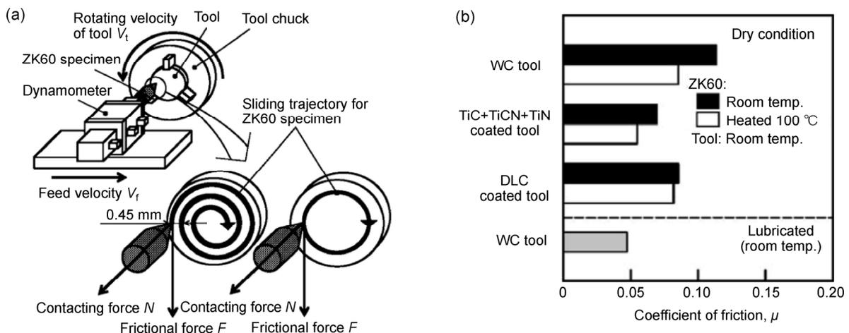
**Fig. 22** (a) Schematic of spiral sliding test on lathe; (b) coefficient of friction of magnesium alloy sliding spirally on surfaces of WC and coated tools. Reproduced with permission from Ref. [58]. Copyright Elsevier, 2014.
