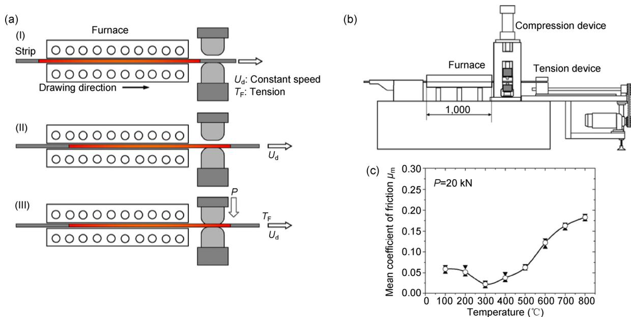
**Fig. 10** (a) Schematic representation of hot flat strip drawing test; (b) schematic representation of hot flat strip drawing test machine; (c) effect of temperature on coefficient of friction. Reproduced with permission from Ref. [77]. Copyright Elsevier, 2014.
