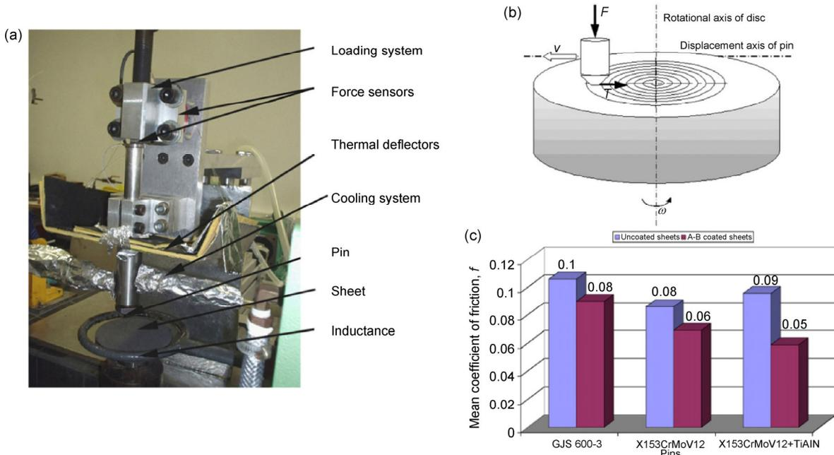
**Fig. 5** (a) Tribometer at high temperature in open contact; (b) pin-on-disc test; (c) mean coefficients of friction after tests at 400 °C. Reproduced with permission from Ref. [73]. Copyright Elsevier, 2014.
