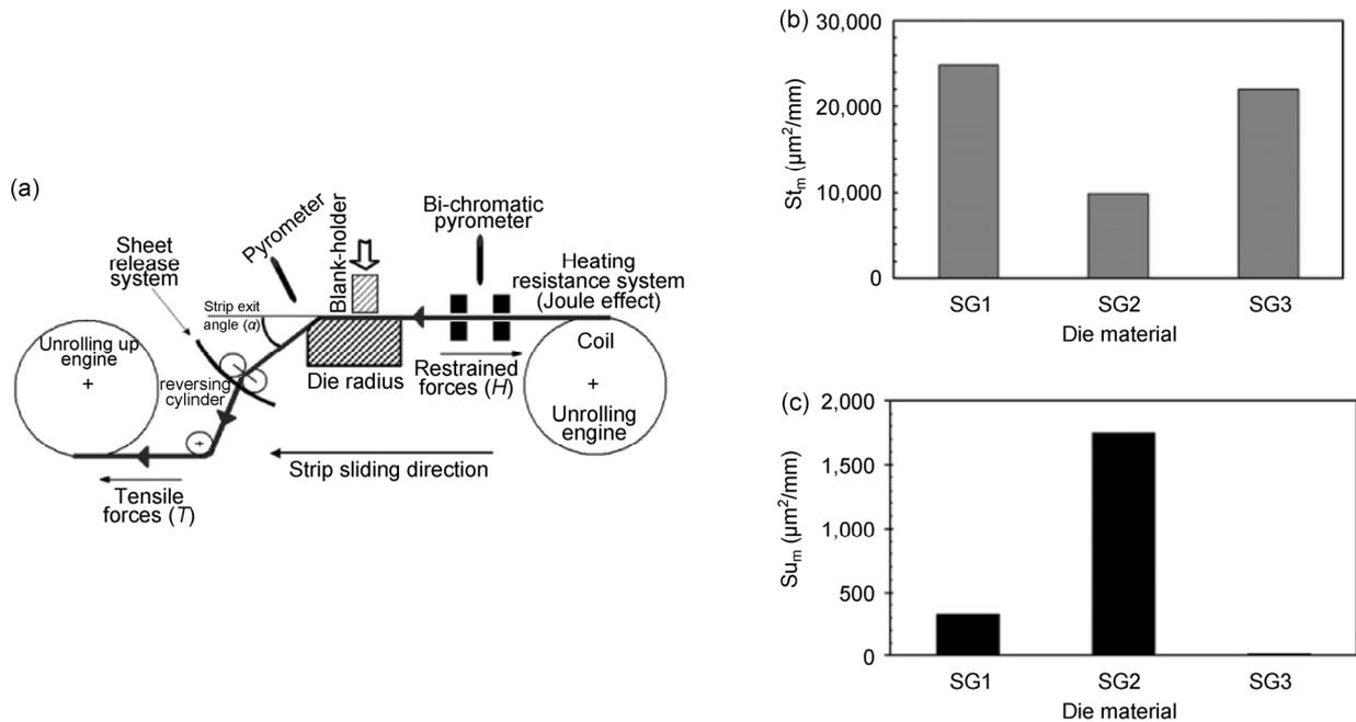
**Fig. 12** (a) Diagram of the deep-drawing process simulator (DDPS); ranking of the three steel grades regarding their propensity to adhesion and abrasion, evaluated respectively by (b) the transfer damage criterion and (c) the material loss criterion after 5,000 cycles. Reproduced with permission from Ref. [39]. Copyright Elsevier, 2015.
