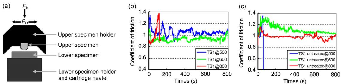
**Fig. 6** (a) SRV test configuration; (b) coefficient of friction vs. time of plasma nitride tool steel 1 and boron steel pair; (c) coefficient of friction vs. time of untreated tool steel 1 and boron steel pair (load: 20 N; stroke 2 mm; frequency: 50 Hz). Reproduced with permission from Ref. [34]. Copyright Elsevier, 2014.
