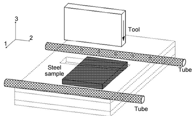
**Fig. 1** Schematic diagram of a chamber showing the positions of the steel sample, the tubes that feed gas and the upper tool. The compression direction (3) is indicated. Reproduced with permission from Ref. [17]. Copyright Elsevier, 2014.
