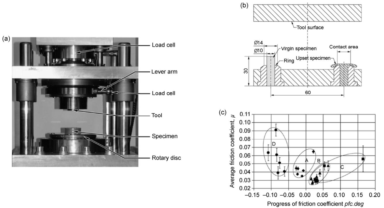
**Fig. 25** (a) The rotational forging tribometer testing device; (b) schematic of the experiment; (c) average friction coefficients of lubricants (A, B, C, and D represent different lubricants). Reproduced with permission from Ref. [60]. Copyright Elsevier, 2014.
