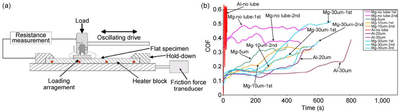
**Fig. 9** (a) Schematic drawing showing the reciprocating tribo- test machine; (b) friction coefficient results of Al 5083 and Mg AZ31B with lubrication for sheet at 450 °C, 50 N load and 0.11 Hz sliding speed with different BN lube thickness. Reproduced with permission from Ref. [76]. Copyright Elsevier, 2014.
