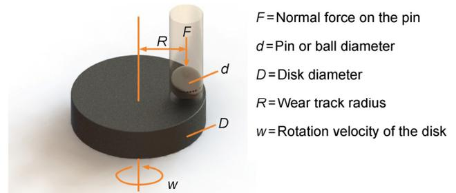
**Fig. 3** Schematic of pin-on-disc wear test system.
