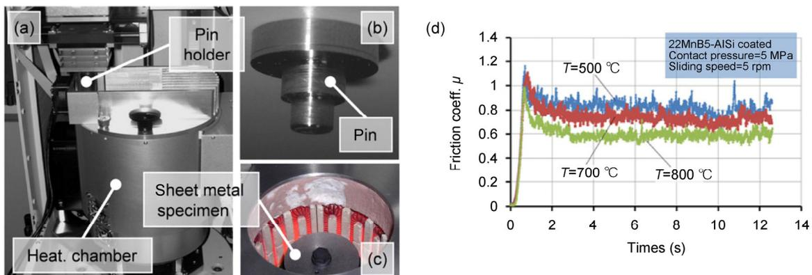
**Fig. 7** High temperature pin-on-disc apparatus: (a) overall experimental setup; (b) pin; (c) disc in the chamber; (d) friction coefficient vs. time at different temperatures. Reproduced with permission from Ref. [74]. Copyright Elsevier, 2014.
