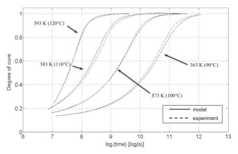
Fig. 7. Validation of Kamal–Sourour model using isothermal curing: degree of cure vs. log(time).
