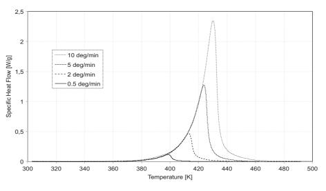
Fig. 4. Total heat of polymerization obtained at different heating rates.
