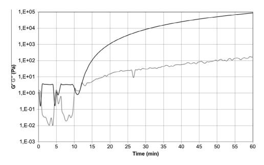
**Fig. 10.** Example of G'/G'' vs. time plot for the isothermal test performed at 100 °C. The rheological tests were designed to monitor the high viscosity range and the results must not be considered before 12 min in this figure.
