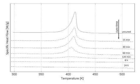
Fig. 3. DSC scans between 293 K (20 °C) and 523 K (250 °C) after different isothermal cures at 383 K (110 °C): residual heat of reaction of the system ( $\Delta H_{res}$ ).
