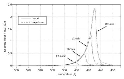
Fig. 9. Dynamic validation of the global Kamal–Sourour model: heat flow vs. temperature.
