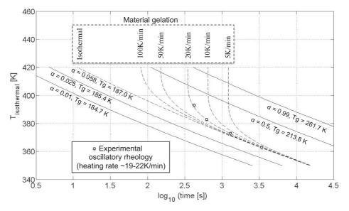
Fig. 12. Isothermal and pseudo-isothermal (100 K/min, 50 K/min, 20 K/min, 10 K/min, 5 K/min) TTT diagrams for the polysilazane system PSZ20 with 1 wt% of dicumyl peroxide. Grey points are the experimental results obtained during oscillatory rheology tests at 363 K, 373 K, 383 K and 393 K.
