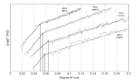
Fig. 11. Loss moduli vs. degree of cure for different isothermal conditions, according to Kamal-Sourour global model and to oscillatory rheology tests.
