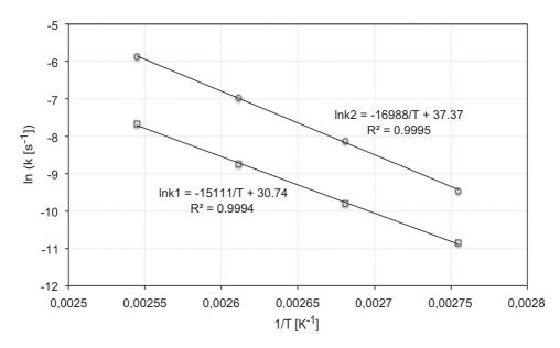
Fig. 6. Arrhenius plots of the two rate constants of the system, according to a Kamal-Sourour model.
