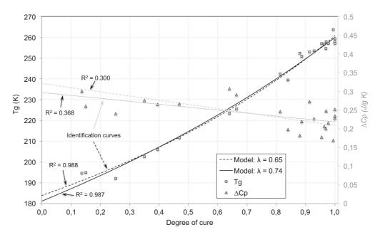
**Fig. 5.** Di Benedetto's plots for the system ( $T_g$  and  $\Delta C_p$ ), using a  $\lambda$  of 0.65 and 0.74.
