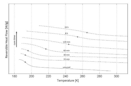
**Fig. 2.** DSC scans between 183 K ( $-90 \degree$ C) and 293 K ( $20 \degree$ C) after different isothermal cure at 383 K ( $110 \degree$ C): glass transition temperature of the system (Reversible Heat Flow). The symbol + shows the  $T_g$  location at each cure time.
