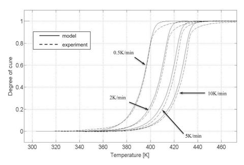
Fig. 8. Dynamic validation of the global Kamal-Sourour model: degree of cure vs. temperature.
