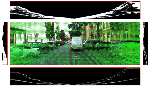
FIGURE 3: The u -velocity before and after thresholding (top, bottom respectively) and the v -velocity before and after thresholding (left, right respectively) represent voting spaces corresponding to the optical field computed (middle) for an image sequence from the KITTI dataset.
