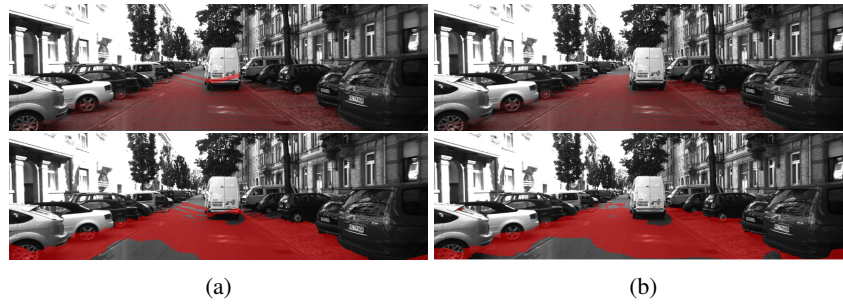
FIGURE 6: Horizontal plane detection based on the c-velocity voting space (a) and v-velocity voting space (b) using the optical flow ground truth (top) and an estimated optical flow (bottom)
