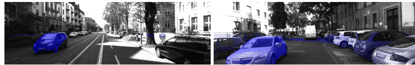
FIGURE 8: Obstacle detection based on the v-velocity voting space using the optical flow ground truth
