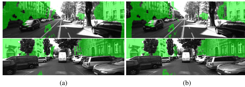
FIGURE 7: Lateral planes detection whenever they are available on image based on the c-velocity voting space (a) and v-velocity voting space (b) using the estimated optical flow
