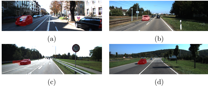
Figure 6: Moving object segmentation on the KITTI "Scene Flow Evaluation 2015 benchmark". Sub-figures (a),(b) and (c) display three segmentation examples, the detected moving pixels are drawn in red. In (a), the moving car has been well detected. In (b), the black one right in front of the camera has not been detected because the car locates nearly at the point of epipole. In (c), some background pixels have been detected as moving due to the occlusion in the next frame. In (d), the silvery car has not been detected because it is out of the detection range.
