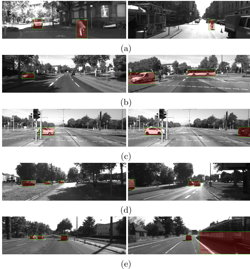
Figure 7: Moving object detection on different sequences. Sub-figures (a), (b), (c), (d) and (e) display the detection results, respectively on sequences 05, 11, 17, 51 and 56 in the category of "City" in the raw data.
