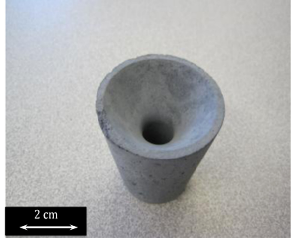
Fig. 2. SiC-based micro-concrete nozzle after manufacturing.
