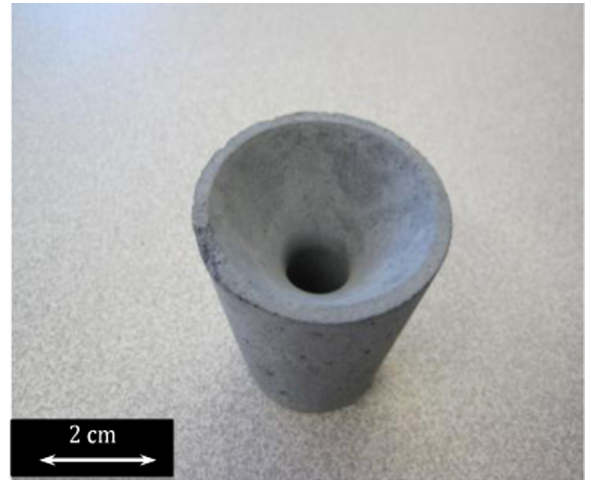
Fig. 2. SiC-based micro-concrete nozzle after manufacturing.
