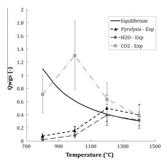
**Fig. 5.** Water-gas-shift constants from pyrolysis, H<sub>2</sub>O and CO<sub>2</sub>-experiments and at thermodynamic equilibrium as a function of temperature.
