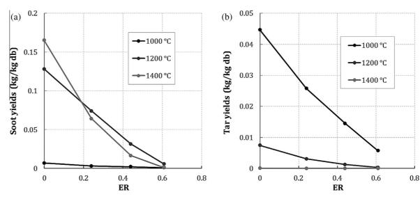
Fig. 11. Soot (a) and tar yields (b) calculated with GASPAR as a function of ER at different temperature.
