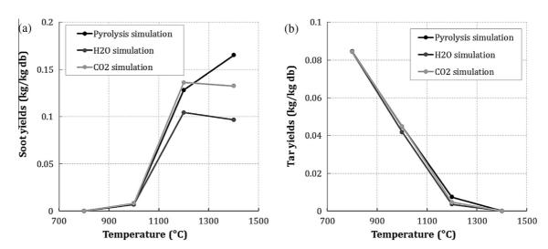
$\textbf{Fig. 6.} \ \ Soot\ yields\ (a)\ and\ tar\ yield\ (b)\ as\ a\ function\ of\ different\ temperature\ calculated\ with\ GASPAR\ in\ pyrolysis,\ H_2O\ and\ CO_2-experiments.$
