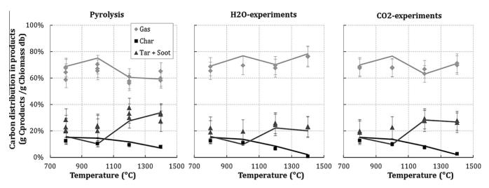
Fig. 3. Carbon distribution in gas, char and tar + soot in pyrolysis, H<sub>2</sub>O and CO<sub>2</sub>-experiments - experimental results (dots) and simulation results (lines).
