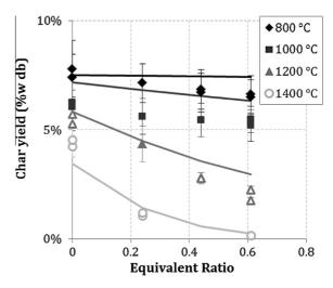
**Fig. 8.** Char yields as a function of ER at 800, 1000, 1200 and  $1400\,^{\circ}\text{C}$  – experimental results (dots) and simulation results (lines) – char ash content measured in furnace (full dots) and in TGA (empty dots).
