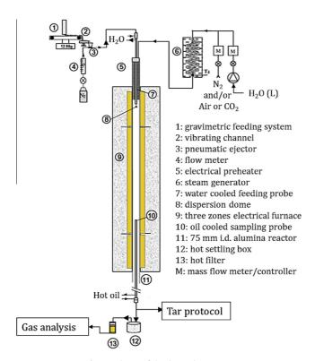
Fig. 1. Scheme of the drop tube reactor.
