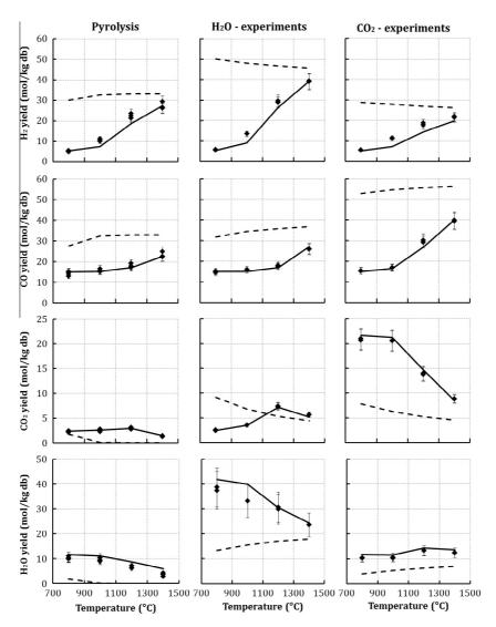
Fig. 4. H<sub>2</sub>, CO, CO<sub>2</sub> and H<sub>2</sub>O yields as a function of temperature in pyrolysis, H<sub>2</sub>O and CO<sub>2</sub>-experiments – experimental results (dots), simulation results (continuous lines) and thermodynamic equilibrium results (dotted lines).
