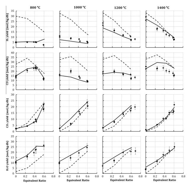
Fig. 9.  $H_2$ , CO, CO<sub>2</sub> and  $H_2$ O yields as a function of ER at 800, 1000, 1200 and 1400 °C – experimental results (dots), simulation results (continuous lines) and thermodynamic equilibrium results (dotted lines).
