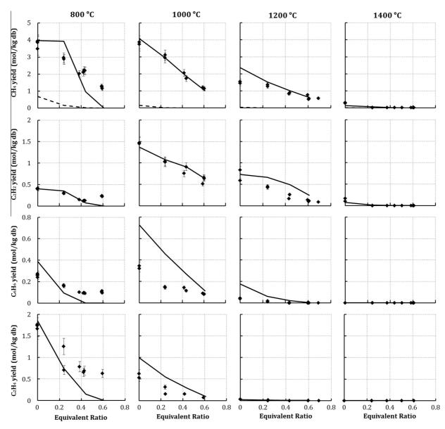
Fig. 10. CH<sub>4</sub>, C<sub>2</sub>H<sub>2</sub>, C<sub>6</sub>H<sub>6</sub> and C<sub>2</sub>H<sub>4</sub> yields as a function of ER at 800, 1000, 1200 and 1400 °C – experimental results (dots), simulation results (continuous lines) and thermodynamic equilibrium results (dotted lines).
