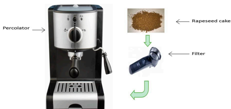
Figure 12. Percolation extraction of proteins from rapeseed cake.
