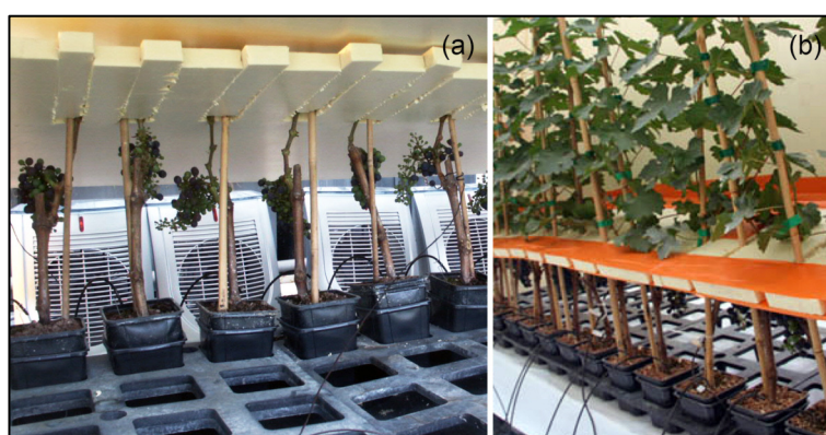
Figure 1 - Experimental system used to investigate the effect of heat at the bunch level. (a) Cabernet Sauvignon fruiting cuttings were used to expose clusters to an elevated T° airflow produced by fan heaters. (b) The other plant organs were all protected from the warmed airflow by polystyrene foam deflectors.
