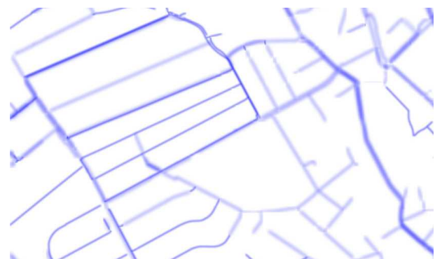
Figure 4: Blurring: different levels of positional accuracy are denoted by different levels of blurring.
