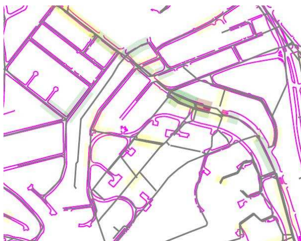
Figure 6: Colour bands showing positional confidence for sewer pipes. Note that not all assets on the map have uncertainty information associated with them.
