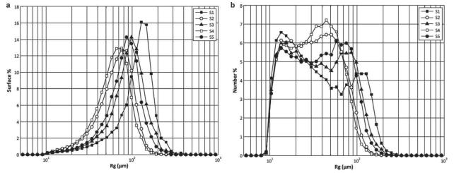
Figure 4. (a) Surface-based gyration radius distributions for the different steps-Run 2 ( $\langle G \rangle$ =190 s<sup>-1</sup>). (b) Numberbased gyration radius distributions for the different steps-Run 2 ( $\langle G \rangle$ =190 s<sup>-1</sup>).
