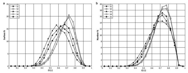
Figure 7. (a) Surface-based circularity distributions for the different steps ( $\langle G \rangle = 190 \text{ s}^{-1} - \text{Run } 2$ ). (b) Number-based circularity distributions for the different steps ( $\langle G \rangle = 190 \text{ s}^{-1} - \text{Run } 2$ ).
