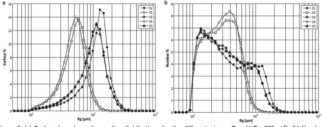
Figure 3. (a) Surface-based gyration radius distributions for the different steps-Run 1( $\langle G \rangle$ =280 s<sup>-1</sup>). (b) Numberbased gyration radius distributions for the different steps-Run 1 ( $\langle G \rangle$ =280 s<sup>-1</sup>).
