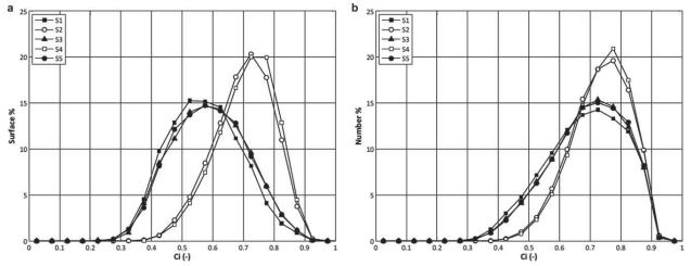
Figure 6. (a) Surface-based circularity distributions for the different steps ( $\langle G \rangle = 280 \text{ s}^{-1} - \text{Run 1}$ ). (b) Number-based circularity distributions for the different steps ( $\langle G \rangle = 280 \text{ s}^{-1} - \text{Run 1}$ ).
