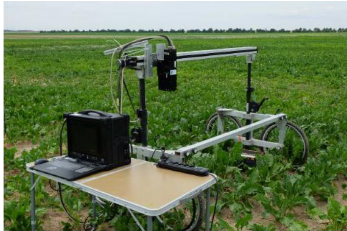
Figure 2: Ground-based platform used for hyperspectral measurements
