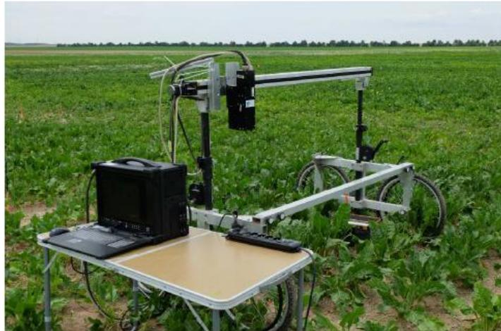
Figure 2: Ground-based platform used for hyperspectral measurements
