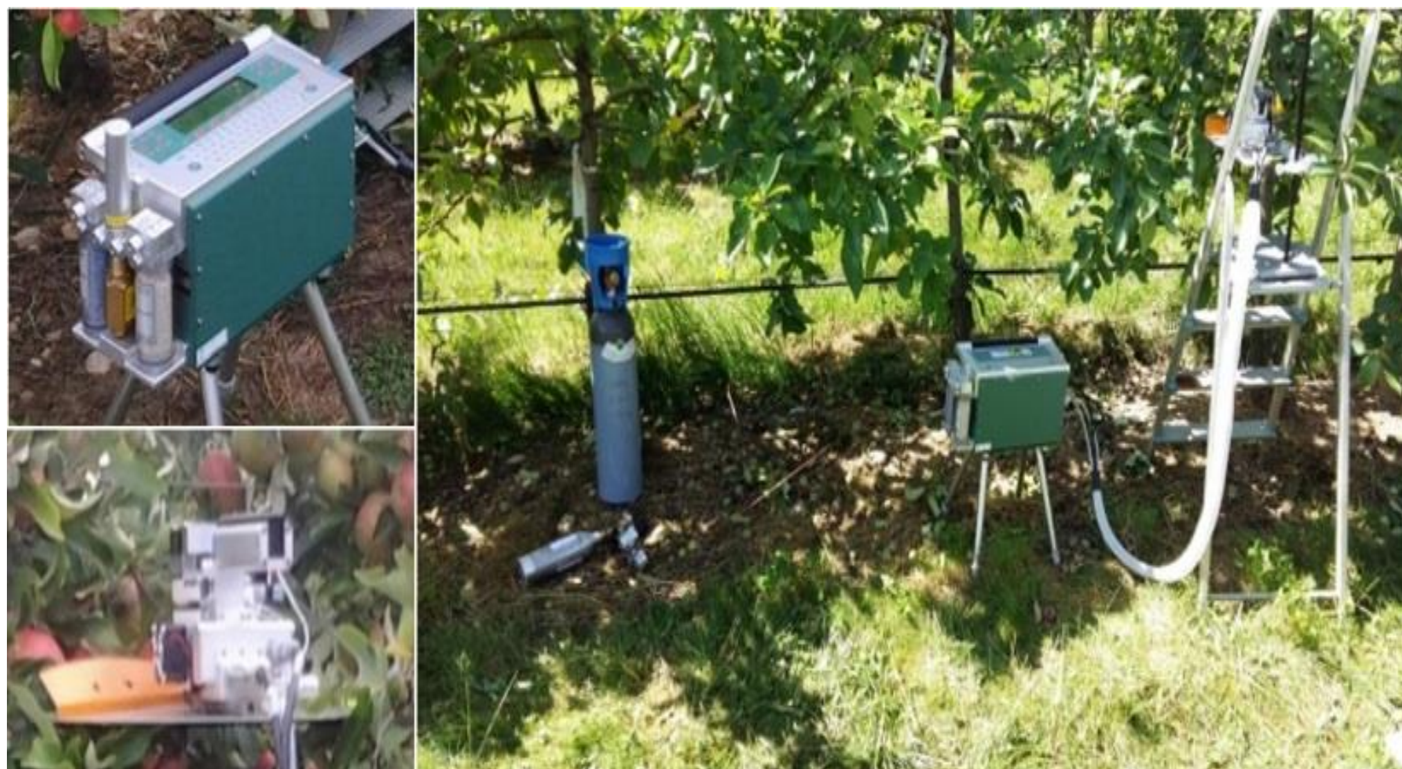
Fig. 1 Experiments used to follow C transport in the branch of apple tree: 13 CO 2 labelling with LI-6400XT portable photosynthesis system.
