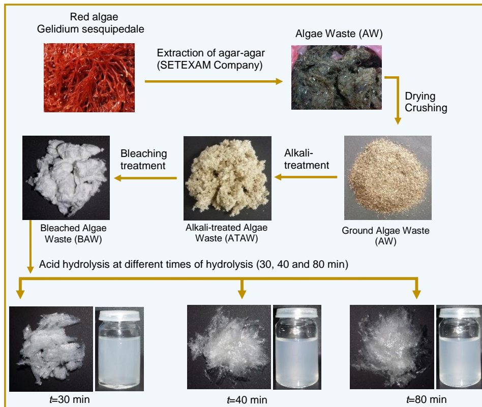
Figure 1: Overall steps of CNC extraction at different hydrolysis times and digital images of each obtained products
