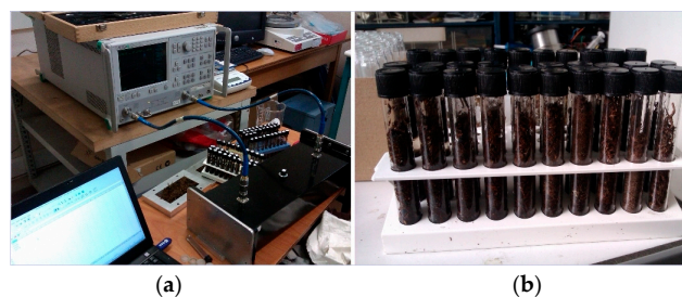
Figure 1. (a) Rectangular resonant cavity with a sample in a glass tube inserted in the center, connected to vector network analyzer (ANRITSU 37325A) by means of two coaxial cables; (b) glass tubes filled with samples of organic material at different wetness contents.
