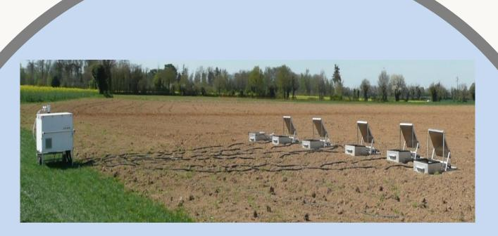
Mobile spectrometers are under development to provide advanced equipments to characterize soil biological activity. Two mobile trailers are setup comprising each instruments to measure in real time the evolution of CO2, H2O, N2O and CH4 fluxes and their isotopic signatures (13C, 15N) on various ecosystems. In addition, a PTR-MS will be conditioned to measure in situ COV emission from soil.
