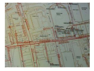
Figure 2: A single-domain service plan showing gas assets in red.
