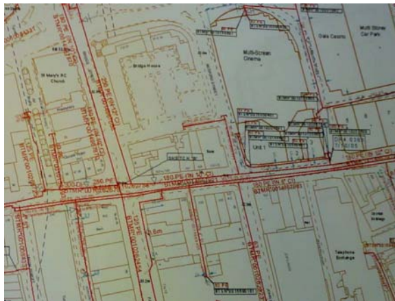
Figure 2: A single-domain service plan showing gas assets in red.
