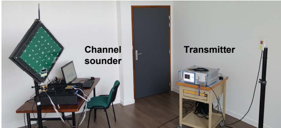
Fig. 11 : Wideband channel sounder measurement setup
