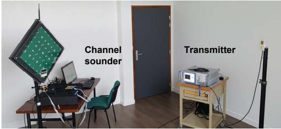
Fig. 11 : Wideband channel sounder measurement setup
