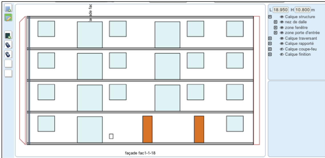
Fig. 3 Façade: frames and load bearing areas
