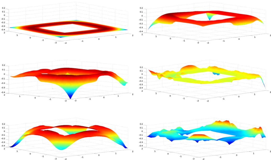
Figure 3 – Test case (a): Six first POD modes.
