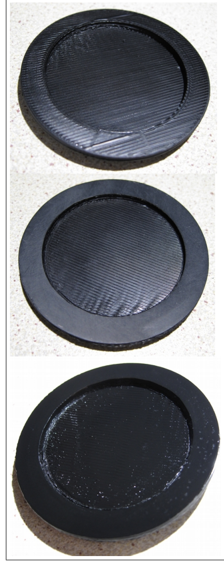
Figure 2: Typical test-samples after printing (top), after polishing with fine sandpaper (middle) ready for testing. Same sample with a Vacseal® varnish coating (bottom) giving a glossy finish (after baking, see IV).
