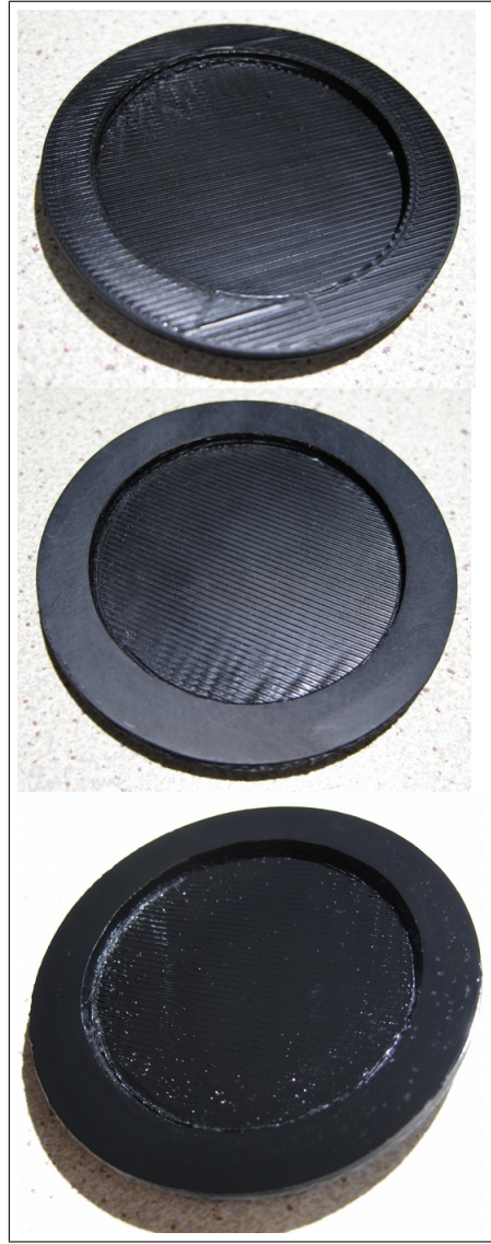
Figure 2: Typical test-samples after printing (top), after polishing with fine sandpaper (middle) ready for testing. Same sample with a Vacseal® varnish coating (bottom) giving a glossy finish (after baking, see IV).
