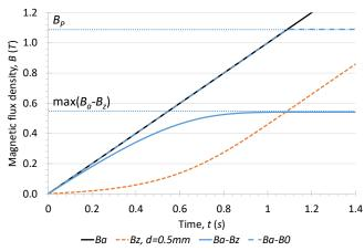
Fig. 5. Numerical calculation of  $B_a(t)-B_z(d=0.5\text{mm}, t)$  and  $B_a(t)-B_0$ , with n = 15,  $V_b = 1\text{T/s}$ .
