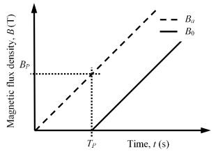
Fig. 2. Linearly growing applied magnetic field  $(B_a)$  and theoretical magnetic field  $(B_o)$  at the center of the pellet versus time (t).
