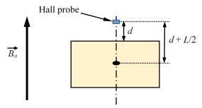
Fig. 3. Hall probe location above the HTS pellet.
