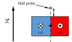
Fig. 6. Complete penetration of the current density with CSM.
