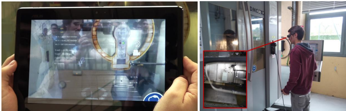
Fig. 2. AR system in operation (on the left: using a tablet PC; on the right: using AR glasses with a zoom on displayed information)
