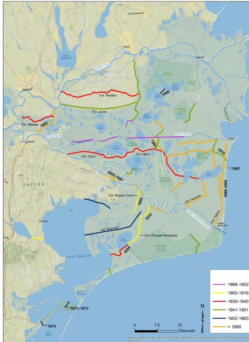
Figure 2. Chronology of the hydro-technical works in the Danube Delta during the 1900-1994 period. The most important canals built during this period: Dunavat (initially called Regele Carol I) in 1907; Dranov (Ferdinand Canal) between 1912 and 1914, which connects the Sfantu Gheorghe Canal to the Razin-Sinoe Complex; Enisala (Elisabeta Canal) in 1913; Litcov (Carol II Canal) between 1929 and 1932; Crasnicol (Voeivodul Mihai Canal) between 1930 and 1934; Sireasa, parallel to the Sulina Branch connecting the Sontea-Furtuna Complex to the Danube branch
