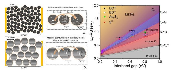
Figure 4 a. Scheme of a film of small HgSe CQDs and of the transition between two resonant states according to Mott VRH. b. Scheme of a film of large HgSe CQDs and of the transition between two CQDs. In ES VRH, electron transfer must overcome the Coulomb energy. c. Fermi energy with respect to the valence band as a function of the interband gap. The solid lines correspond to the mid interband gap,  $1S_e$ ,  $1P_e$  and  $1D_e$  states from the 3 band  $k \cdot p$  simulation.
