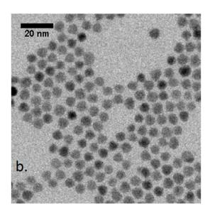
Figure 1 a. Absorption spectra for four sizes of HgSe CQD. b. TEM image of medium size HgSe CQD.
