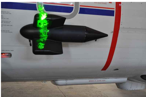
FIG. 4 ALIDS tests on the ground after integration on the ATR-42.
