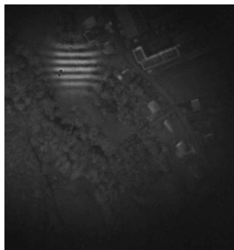
FIG. 5 Examples of ILIDS images obtained in clouds during the flight test.
