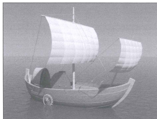
Figure 3. Vitruvius's maritime odometer (1 st century BC).
