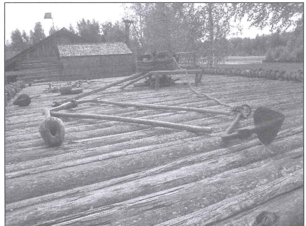
Figure 7. Horse-powered raft for floating wood in Finland, 20 th century.
