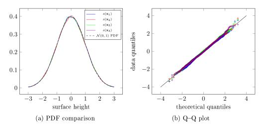
Figure 3: Verification of surface height distribution in four points on the surface
