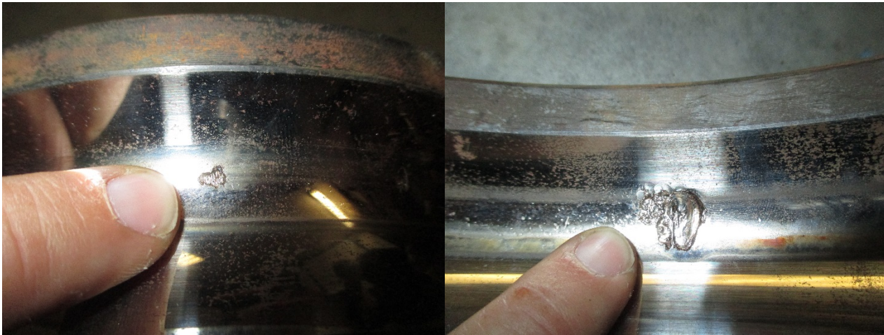
Figure 4: inner ring defect (on the left) and outer ring defect (on the right) of the generator front bearing.
