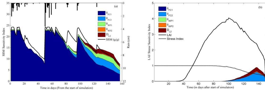
Figure 7: Temporal variations of (non-normalized) Sobol' main sensitivity indices of (a) SSM and (b) LAI to soil hydraulic parameters and 2<sup>nd</sup> layer depth during the entire simulation period for one plot of maize crop. Solid black curves represent the mean of simulated (a) SSM and (b) LAI. Bar chart in (b) represents the rainfall (in cm). Dashed black curve in (b) represents the mean of simulated water stress.
