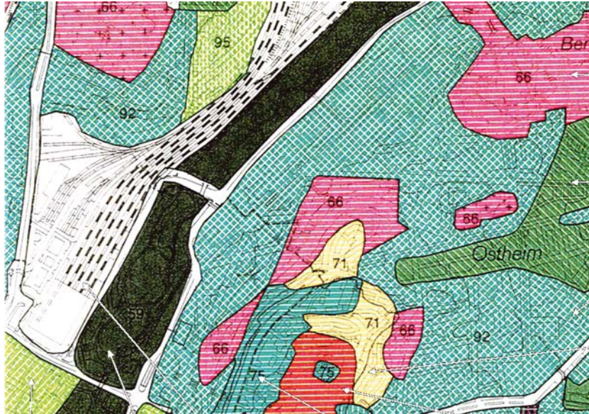
Fig. 5.2-8. Extract of urban soil map of Stuttgart with soil groups Technosol, Regosol, Cambisol and Colluvisol (based on Holland et al. 1997; modified and illustrated). Annotation: Designation of soil group «Colluvisol» according to German soil taxonomy and not in coincidence with WRB soil group (FAO 2014).
