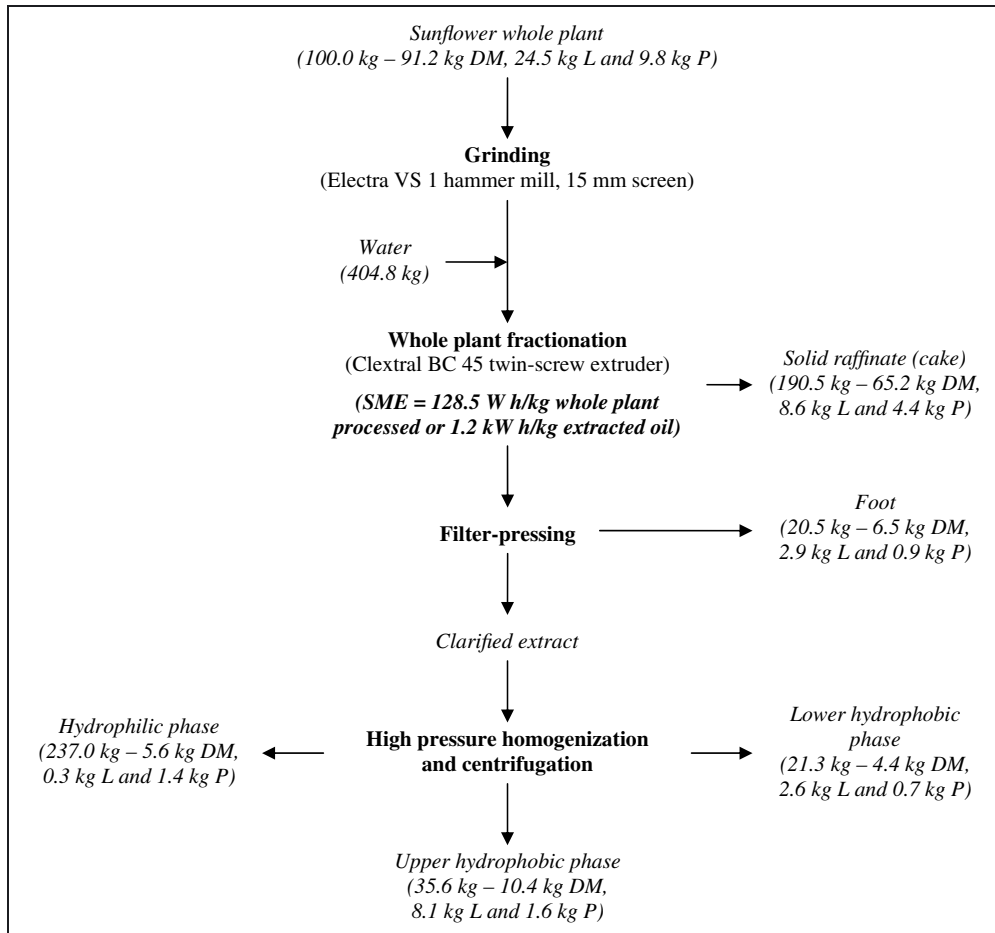
Fig. 5. Assessment of the whole plant fractionation in the twin-screw extruder under the optimal operating conditions (DM, dry matter; L, lipids; P, proteins; SME, specific mechanical energy consumed by the motor).
