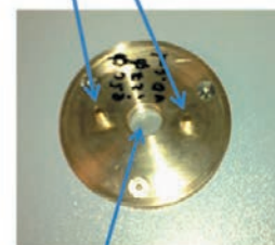
► Starch disk confined between mica sheet
