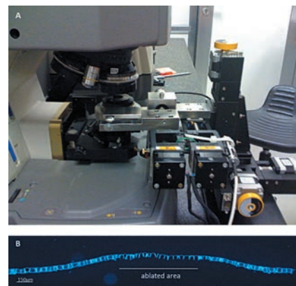
► Figure 1: A) Experimental device on the SMIS microscope. B) Cross section of the aleurone layer placed on the microtensile stage (observation: epifluorescence microscopy under UV light. Blue autofluorescence due to cell wall phenolic compounds).
