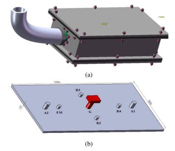
Fig. 1. Multi-sensor bedload transport monitoring platform: (a) general view, (b) setup of the acoustic sensors on the top steel plate.
