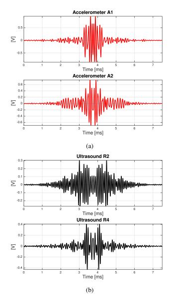
Fig. 2. Sensors recordings in passive configuration, 1 buffer triggered by A1: (a) accelerometers and (b) ultrasound transducers.
