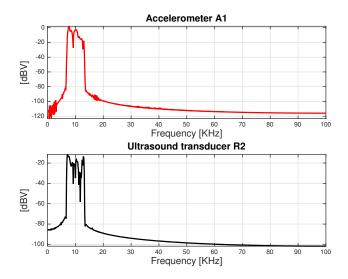
Fig. 3. Sensors recordings spectra in passive configuration, 1 buffer triggered by A1: accelerometer A1 (up) and ultrasound transducer R2 (down).
