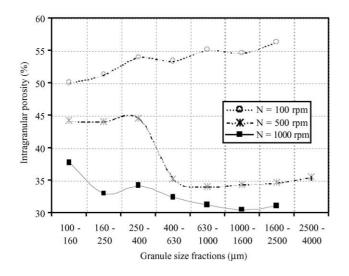
Fig. 8. Shear effect on intragranular porosity of granule size fractions, L/S = 31.7% (w/w), top = 19 min.
