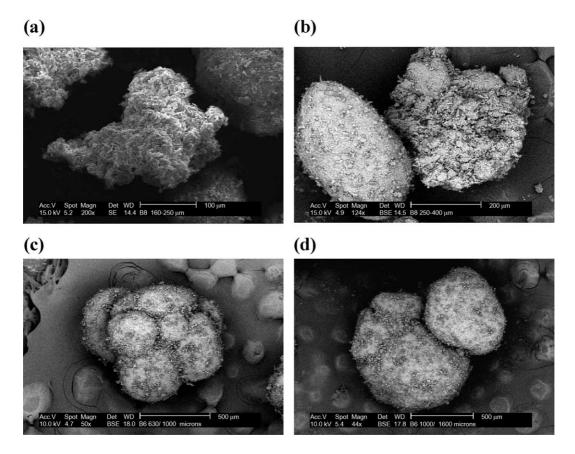
Fig. 5. (a-b) Densification (Regime II), small granules (160–400  $\mu$ m), L/S=31.7%, top=19 min, N=500 rpm. (c-d) Coalescence (Regime II), granules (630–1600  $\mu$ m), L/S=31.7%, top=19 min, N=500 rpm.
