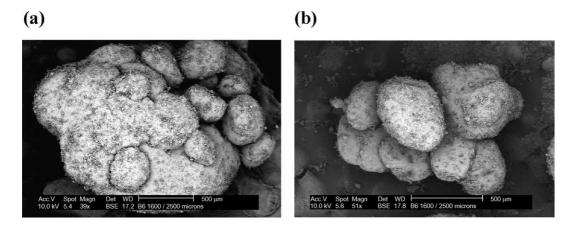
Fig. 6. (a-b) Extensive (Regime III), granules (1600-2500 µm), L/S=31.7%, top=19 min, N=500 rpm.
