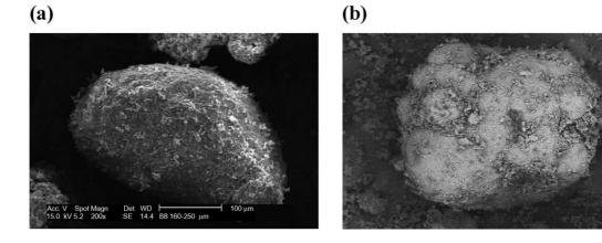
Fig. 4. (a-b) Nucleation, coating and coalescence between nuclei (Regime I), size class (160–250 µm), L/S=31.7%, top=19 min, N=500 rpm.
