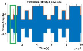
Figure 2. PD+COMM signals (blue) & envelope (red).
