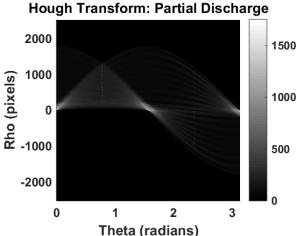
Figure 9. Hough transform of the partial discharge.
