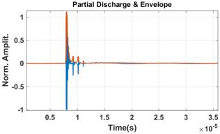
Figure 1. Partial discharge (blue) & envelope (red).
